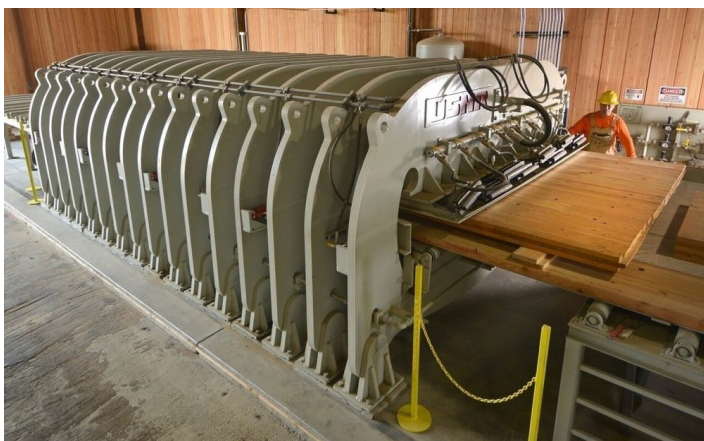
CLT panel being manufactured at DR Johnson Lumber Co in Riddle, Oregon | Source: Lever Architecture
